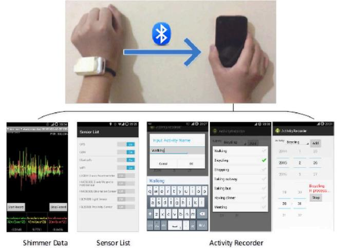
Fig. 3. Devices and applications for data collection and user annotation
